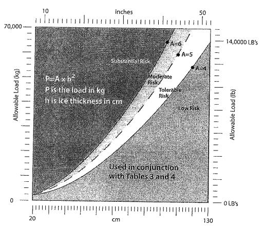
Figure 20 Ice Bearing Capacity Chart
